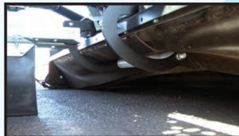
The optional in-cab, operator controlled Pick-Up Head **Front Curtain Lifter** raises the front curtain allowing large amounts of lighter materials, such as leaves, to easily pass beneath the pick-up head.
