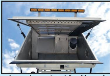
Large, heavy duty 4.0 cubic yard hopper. Hopper, dump door, inspection door, hopper screen and dust separator available in optional non-magnetic, low carbon, high chrome stainless steel for maximum corrosion resistance.
