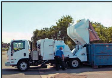
The heavy duty pick-up head utilizes **True Regenerative Air** - a controlled jet of air through the entire width of the blast orifice into pavement cracks forcing up fine dust particles into the air stream. The pick-up head delivers maximum air blast and powerful vacuum across the entire width of the pick-up head allowing for removal of heavy debris, light debris and fine dust.
