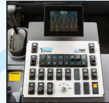
**In-cab controls** are center mounted and illuminated for ease of operation from either driving position. Switches integrate multi-color LEDs giving operators instant feedback on sweeper functions.
