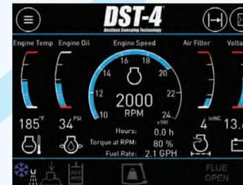
The color touchscreen display delivers **on-board diagnostics** for the TYMCO BlueLogic® Control System and the auxiliary engine's ECU (Engine Control Unit). Service reminders are displayed for the auxiliary engine and hydraulic system fluids and filters.
